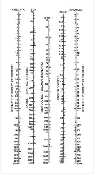
How to use: Place straight edge at equal centistoke values on both Kinematic scales. All viscosities on each scale will be equivalent for the same temperatures. To extend scale ranges to higher viscosities utilize powers of 10 in these scales between the 100 and 1000 divisions on the Kinematic scale. Example: 3000 centistokes = 300 cSt x 10 and is approximately equivalent to 14000 x 10 = 14000 SUS.
