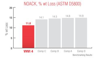
Low volatility is critical in finished formulations for reduced oil consumption and emissions, particularly with increased oil drain intervals and higher engine operating temperatures.
