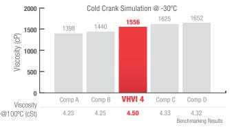
Note: VHVI 4 has a higher Vis @100°C, but a comparable CCS Cold Crank Viscosity measures ease of starting at low temperatures (wear at low temperatures). Lower cranking resistance means faster, easier starting in engine oils.
